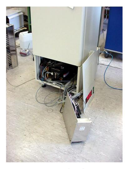
Removed Electronics Module placed it in front of machine. The unit may be operated with the Electronics Module removed. Special care must be taken that cables and connectors are free. Secure workspace and mark area with Danger Sign.
