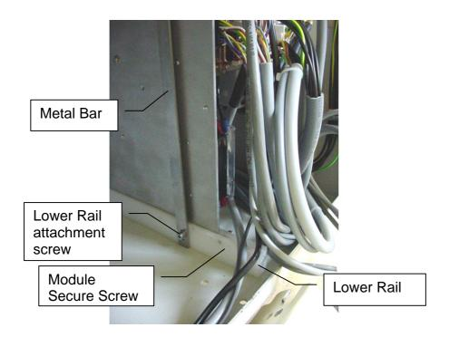
Remove lower rail attachment screws and rotated metal bars aside. Remove Module Secure Screw.
