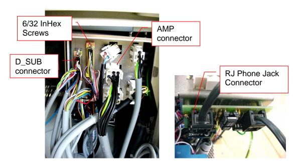
D-SUB connector type and AMP connectors are located on the Connector Panel. All connectors must be removed. One RJ-Phone Jack connector for the serial communication is located on the Electronics Module. Do not forget to remove this connector.
