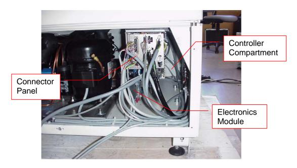
The Electronics Module is located in the Controller Compartment.
