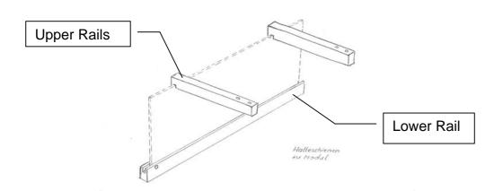
By three rails the Electronic Module is held in place. Two metal bars are attached between the lower and upper rails.
