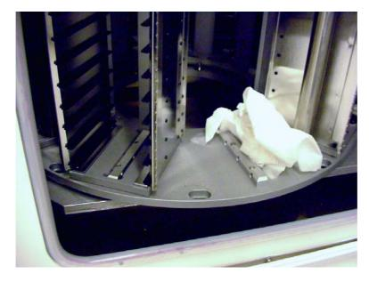
After ~15..30 min. interior reaches room temperature. Dry condense water using a soft cloth.
