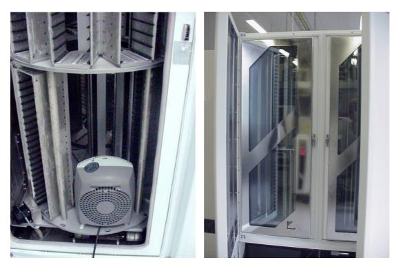
Temperature regulator. Close door after placing heater. To avoid excessive frost inside the chamber do not leave door open. It is important to close door as quickly as possible.
