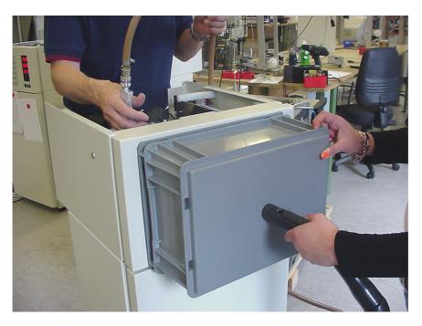
Direct compressed air jet for maximum cleaning effect. The cleaning effect results from the compressed air blowing directly on the condenser surface. Direct jet over entire surface of condenser at small distance.
