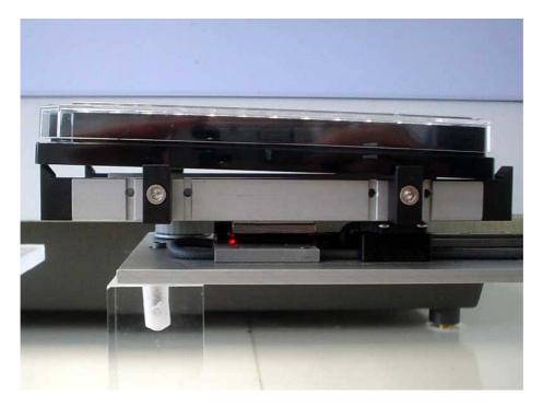
The inner position of the Slide Station is to close to the back plane or the Gate Most likely the machine was pushed inwards.
