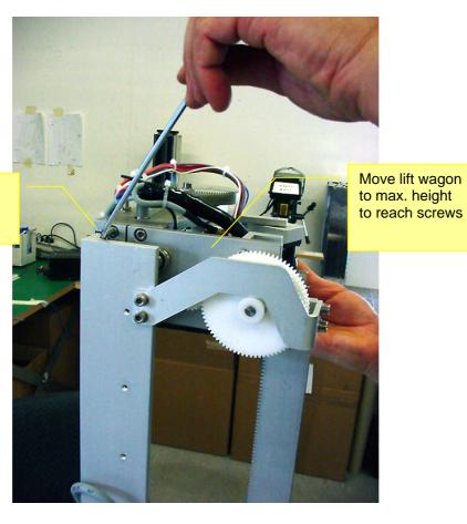
Tighten horizontal lift plate screws
