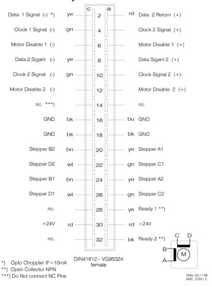
Data (+) lines are connected to +24V. Data inputs are low active.
