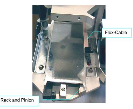
Clean the rack and pinion, Adjust play of the gear by shifting the shovel motor assembly.
