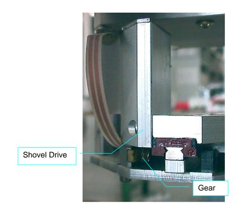
Check if the gear has become lose on the shovel motor axis. The gear is bonded on the motor axis.
