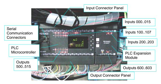
Inputs are numbered as banks 000..400. Each bank has 16 (0..15) maximum. The inputs are located on the top end of the PLC Micro controller. Outputs are numbered 500..900 in banks of max. 16 outputs per bank. The outputs are located on the bottom end of the PLC Micro controller.
