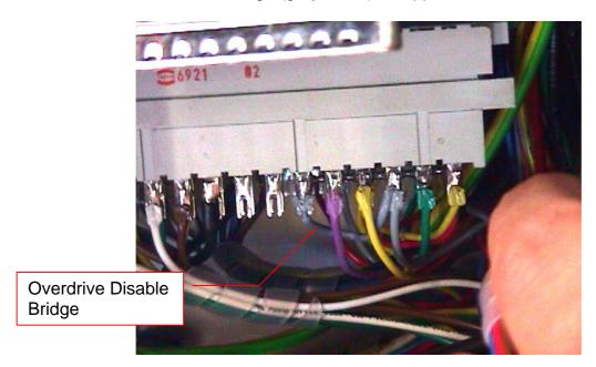
Remove bridge by cutting the grey wire. The picture below shows the connector with Disable Bridge removed.
