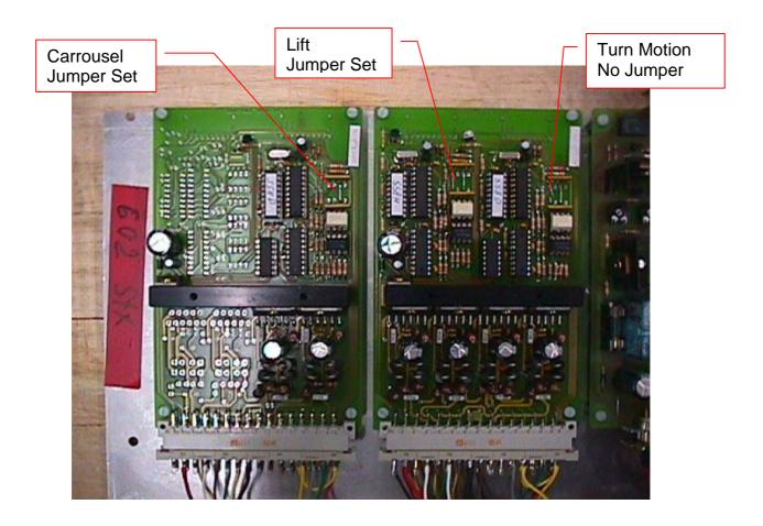
There are four jumpers the jumper at the innermost position is the direction definition. These jumpers are read during start up.
