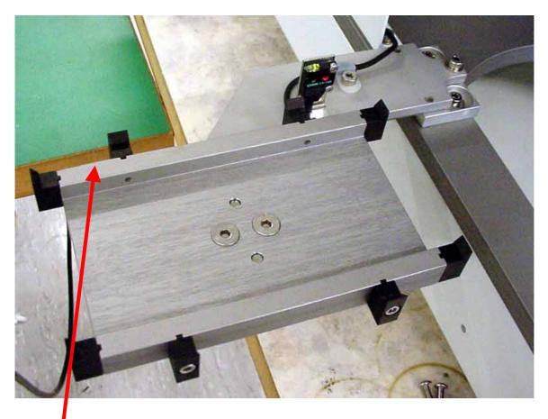
Please have the sensor placed in the location of the Arrow, this is what I did for Astra on the STX 1000 to eliminate the reading of the BCR issue at the transfer station
