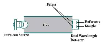
The infrared filter is chosen to ensure that the sensor is totally gas specific and will not exhibit cross sensitivity to other gases.
