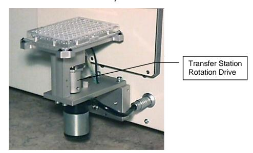
Rotation is controlled by the StoreX system. No additional external software is required.
