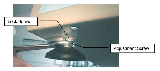
Check that each foot has contact with the ground and that the instruments weight is evenly distributed over all four feet. Allow enough room between the underside and the ground floor. Check rear of instrument for free Gate movement.
