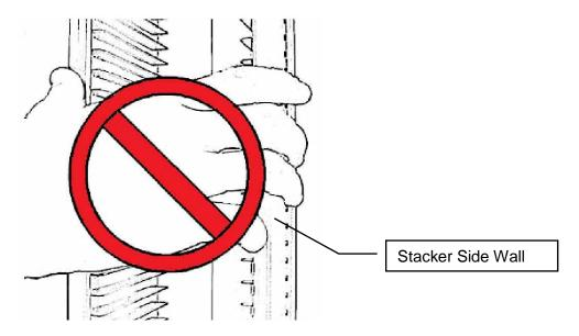
In the rare event of a blockage with the extended shovel in the stacker, the shovel must be carefully pushed backwards until it can move freely, then the stacker can be removed.
