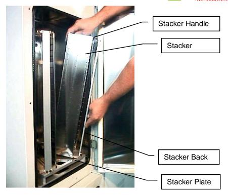
The stackers are secured by alignment rails to the stacker plate. The stackers may be tilted slightly backwards (towards the front opening) for removal. In order to load a stacker align the back of the stacker base plate to the centering pins located on the stacker plate. Push the stacker forward until it stands vertically. The stacker should now stand firmly on the stacker plate. There should be no movement.
