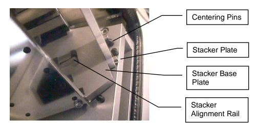
To remove a stacker pull the stacker handle slightly backwards, tilting it, then lift the stacker until it loosens from the stacker alignment rail. Use both hands for this operation. Never use force.
