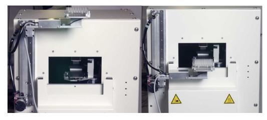
The Lift Station is normaly in upper Position, when Handler loads or unloads a Plate to the Station the station goes to the load Position.
