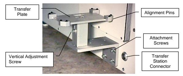
The transfer station can be easily adjusted. The transfer plate can be adjusted horizontally and vertically. Rotation of the transfer plate can also be adjusted.
