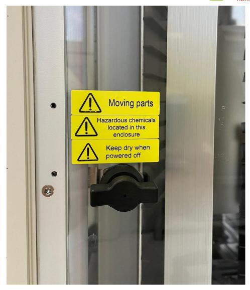
Please be aware that when the unit is powered off, the environment inside the chamber remains static. This could potentially lead to damage to the internal components. It is important to ensure that the unit is properly dried and allowed to reach equilibrium with the room before powering it off. This will help prevent any adverse effects on the system.
