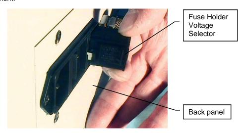
The voltage setting is displayed in a small window in the fuse holder.
