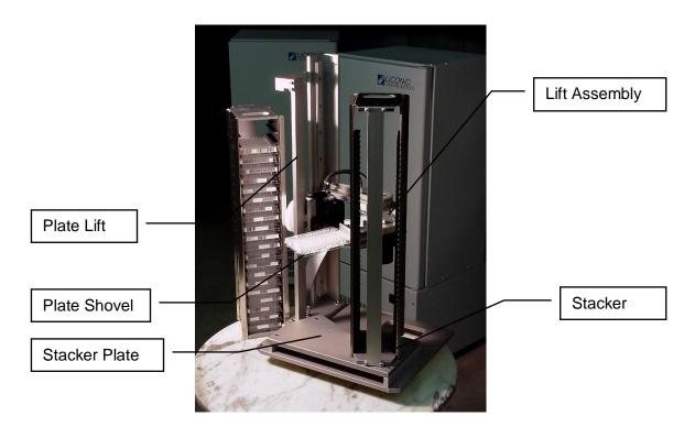
A Handler (4) is used for vertical transport as well as loading and unloading of samples. The Handler consists of a Vertical Positioning Drive (40), a Turn Drive (42) and a Shovel Drive (43). The Handler has a number of vertical positions which are determined by the number of stacker levels and the loading or unloading level.
