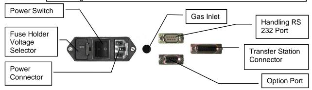
Prior to connecting the instrument to the power source choose the correct voltage setting and the appropriate fuse. The voltage selector is located at the rear of the instrument.
