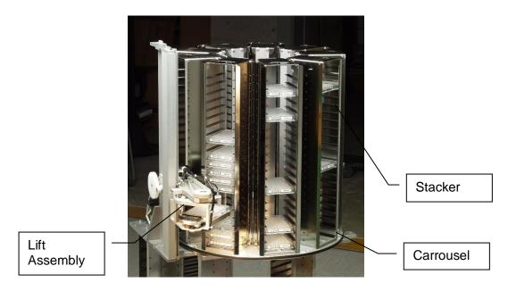
A Handler is used for vertical transport as well as loading and unloading of samples. The Handler consists of a Vertical Positioning Drive, a Turn Drive and a Shovel Drive an a Rotating Drive. The Handler has a number of vertical positions which are determined by the number of stacker levels and the loading or unloading level.
