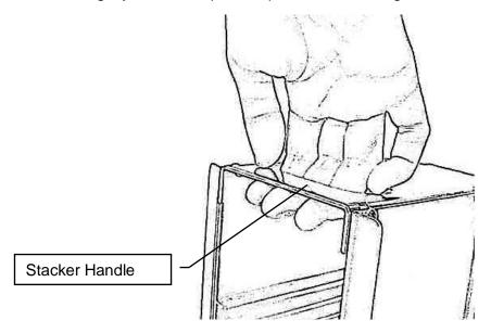
Never apply force to the stackers. Do not drop stackers as Mechanical shock will misalign the stacker. Never lift a stacker by its side walls for this may bend the side walls of the stacker. Bent side walls cause the plates to block when being loaded or unloaded.
