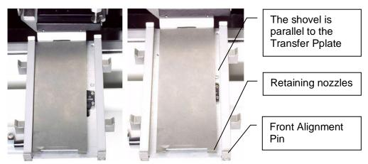
With the shovel extracted you may now adjust the Transfer Station more accurately. The Transfer Plate should be parallel to the Transfer Plate or station?. The two retaining nozzles at the front of the shovel should be parallel to the front edge of the Transfer Plate and behind the two front alignment pins.
