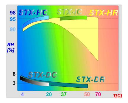
HR-units are Wide Range instruments that cover a wide temperature range. They are a combination, with integrated heater and cooler. Note that all cooled StoreX have an integrated active cooling system. No additional external cooler is needed.
