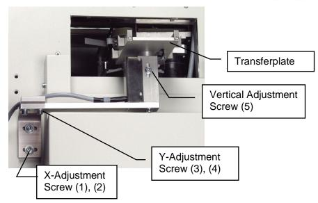
In order to adjust the Transfer Station in the Y-direction (perpendicular to the backplane) use the screws (3) and (4) and slide the Transfer Station into position then tighten screws again. The Height of the Transfer Plate is adjusted by opening screw (5) and lifting or lowering the Transfer Plate. Again, tighten screw (5) after finishing the height adjustment.
