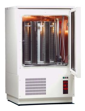
Copper prevents microorganism from growing on the chamber's surface. The disinfections process by copper is rapid and typically starts within minutes. The vast majority of microbes are being killed within less than an hour, while these microbes can survive on a stainless steel surfaces for weeks.
