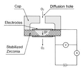
By attaching a cap with an aperture on one side (cathode) of the disc, the gas diffusion is limited and the saturated current is observed. It is termed "limiting current". The limiting current is proportional to the ambient oxygen concentration.
